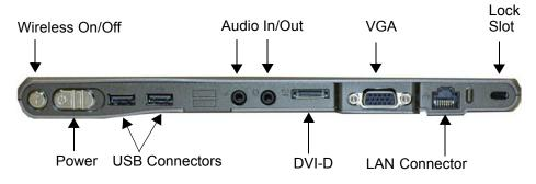
**USB Connectors.** Two USB connectors are included. These can be used to connect any USB device to the Tablet Client.
